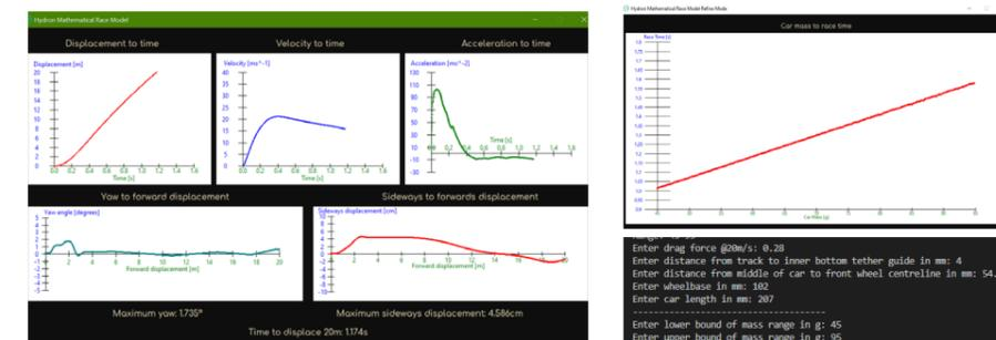
Left: Output data from race model. Right top: Race model refine mode output graph, illustrating direct correlation between increased car mass and increased lap times. Right bottom: Race model refine mode input. Credit: Hydron
