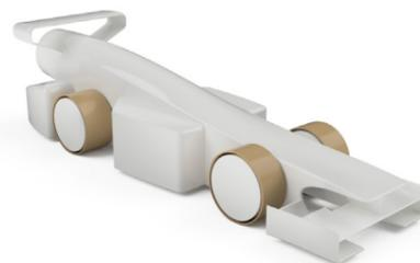
After prototypes A, B, C and D were designed, the key improvement actions were then compiled and were applied to a single combined prototype. The combined prototype took the convex-concave nosecone from our National Finals car, while implementing continuous channel walls along the body for uninterrupted airflow through the central channel. The side pods were slightly tapered to account for the wheels being positioned slightly inwards.
