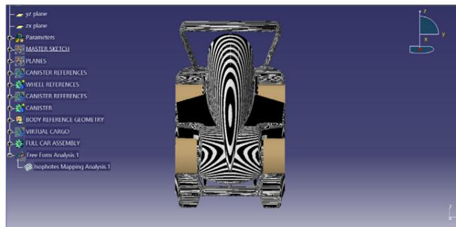
✦ PROTOTYPE-D Isophotes Mapping Analysis - Nosecone and side pod top surfaces are tangential, encouraging airflow over side pods. Credit: Hydron
