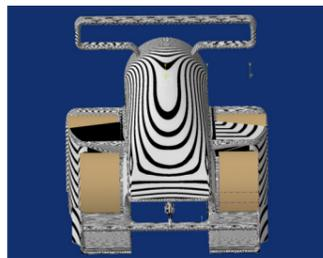
\* Isophotes Curvature Mapping - Tangent Surfaces with no sudden curvature changes. Credit: Hydron
