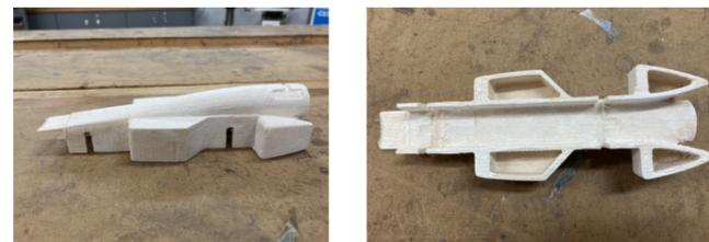
» Test balsa milled car, with machining errors on sidepod and in central tunnel. Credit: Hydron
