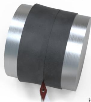
We noticed the problem of a concave thread after the CNC process. We figured out that due to the small wall thickness, the wheels outer surface bent towards the inside while cutting. To solve this issue, a mounting rig was designed to support the wall during turning. These wheels proved to be a major factor in our cars performance.
