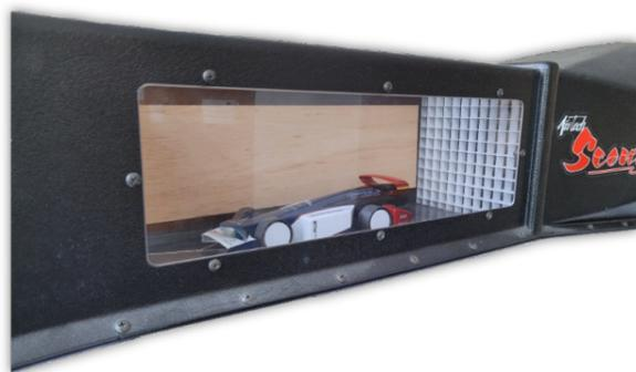
Fig. 3: Real wind tunnel testing (measuring the drag force)
